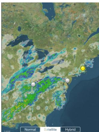
Radar loop details are displayed at the bottom right of the screen in the black bar. The date is shown first followed by a slash and then the beginning and end time of the currently displayed radar loop in Zulu. Current Zulu time is displayed in the center of the black bar for reference The radar imagery is updated automatically as new radar imagery becomes available from NOAA. Tapping the date on the black bar performs a manual check for new radar imagery.
