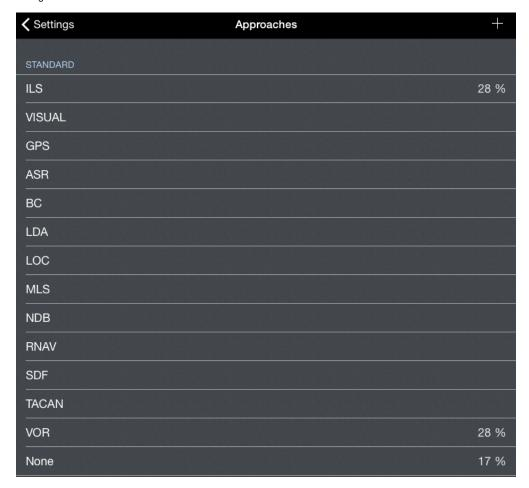
The Approaches page is broken down into two sections. Standard approaches built into APDL are listed together at the top while any custom approaches created are listed separately at the bottom.
